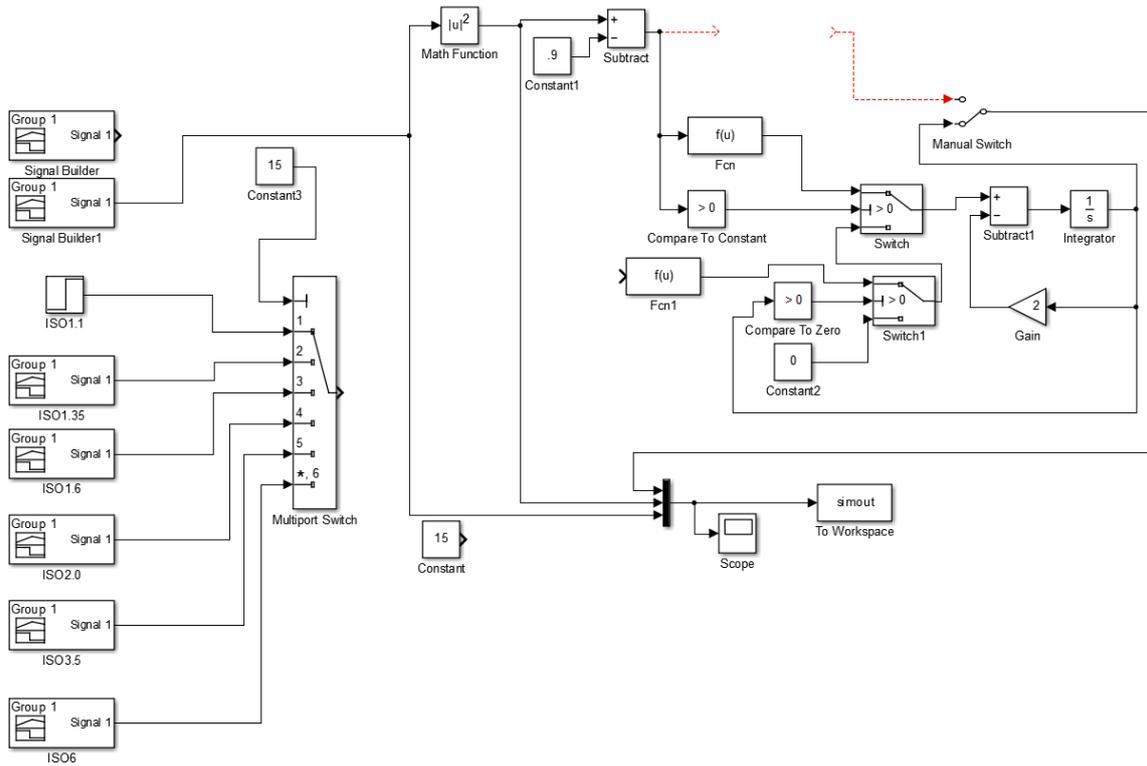
Figure 30: Experiment model for imitating the tripping scheme outlined in ISO 8820-3
