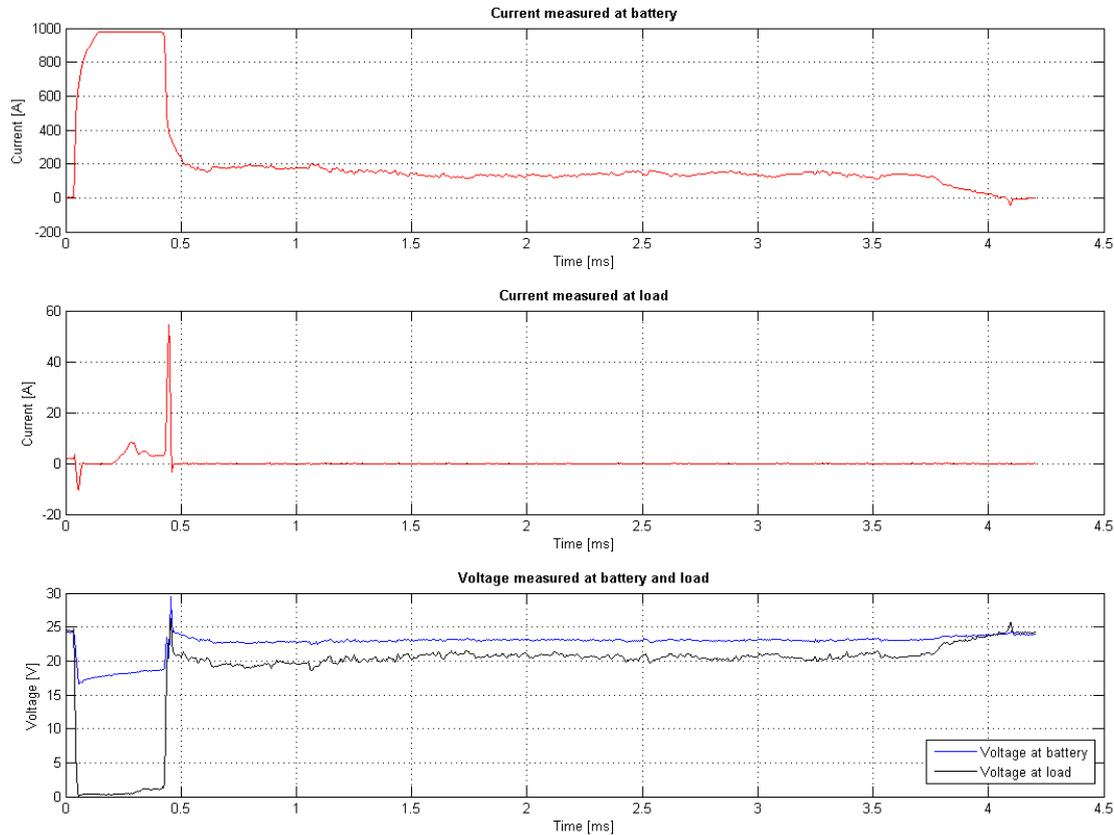
**Figure 21: Currents and voltages typically appearing when squeezing a cable. The pattern was repeated when shaking the cable lightly. It corresponds to a short-circuit to ground during a limited time.**
