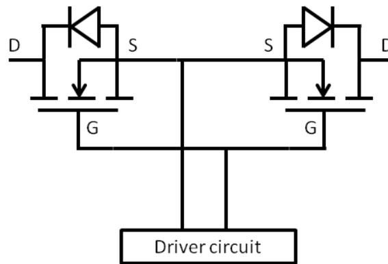
Figure 6: Anti-serial MOSFETs for breaking of regenerative currents
