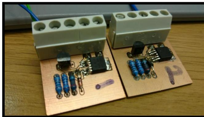
Figure 38: Two modules for evaluating the AUIPS7125RTRL SPS
