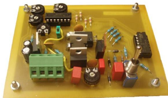
Figure 1: The Active Fuse System prototype built by Sjöberg and Steen in 2008 [2]
