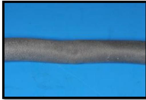
Figure 22: Cable after bending simulation, 1 of 5 samples
