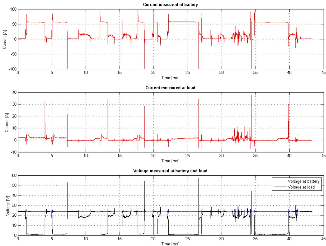
Figure 25: Currents and voltages measured during cutting-simulations
