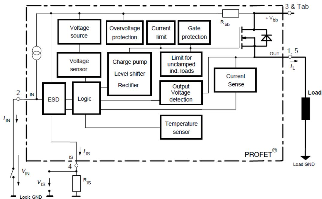
Figure 7: Schematic functional diagram of the Infineon BTS555 [21]
