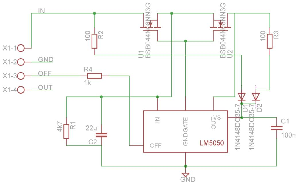
Figure 35: Anti-serial MOSFETs with LM5050 drive circuit. A solution proposed by Jan Hellgren, RECU.
