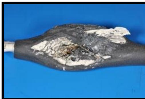
**Figure 20: Cable after squeezing, 1 of 14 samples**
