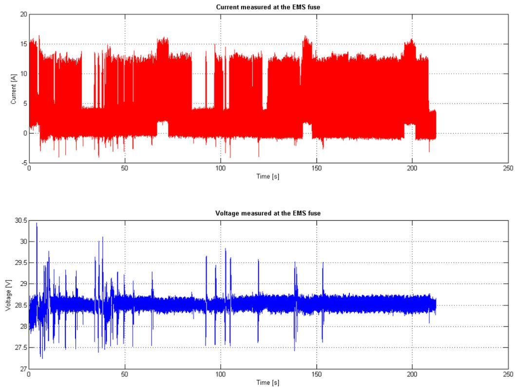
Figure 18: Current and voltage measured on one of the EMS fuses
