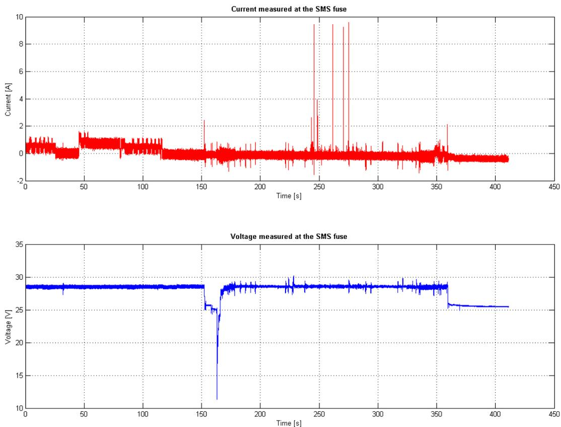
Figure 16: Current and voltage measured at the SMS fuse
