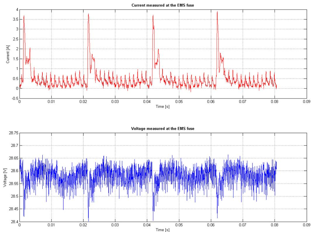
Figure 19: Current pulses from Figure 18
