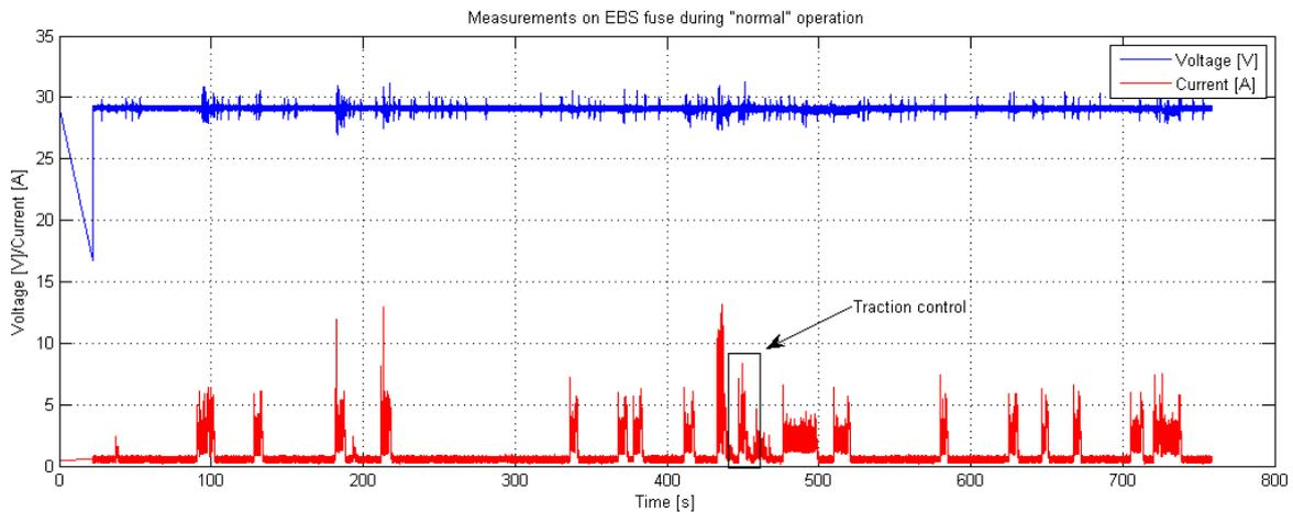
Figure 15: Voltage and current measured at EBS fuse
