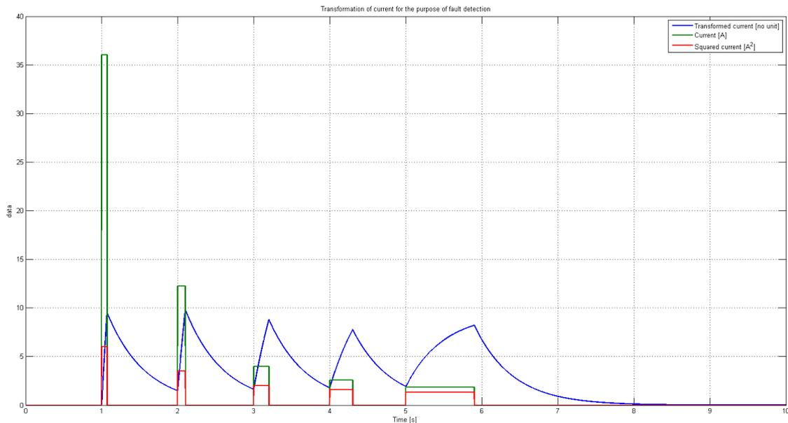
Figure 31: Transform of current test pulses according to ISO 8820-3
