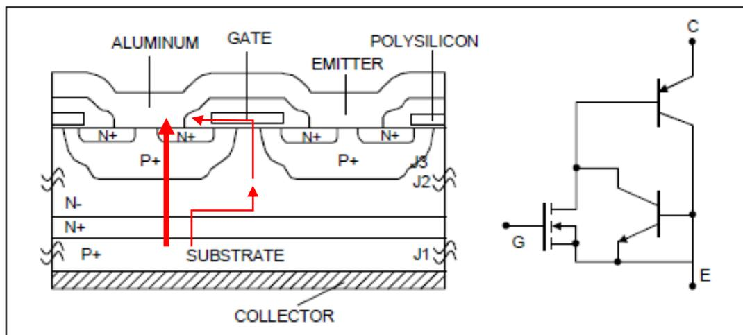
Figure 4: The IGBT structure and equivalent schematic [6]
