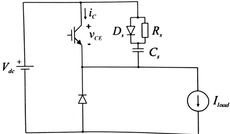
Figure 5: An example of a snubber circuit [6]
