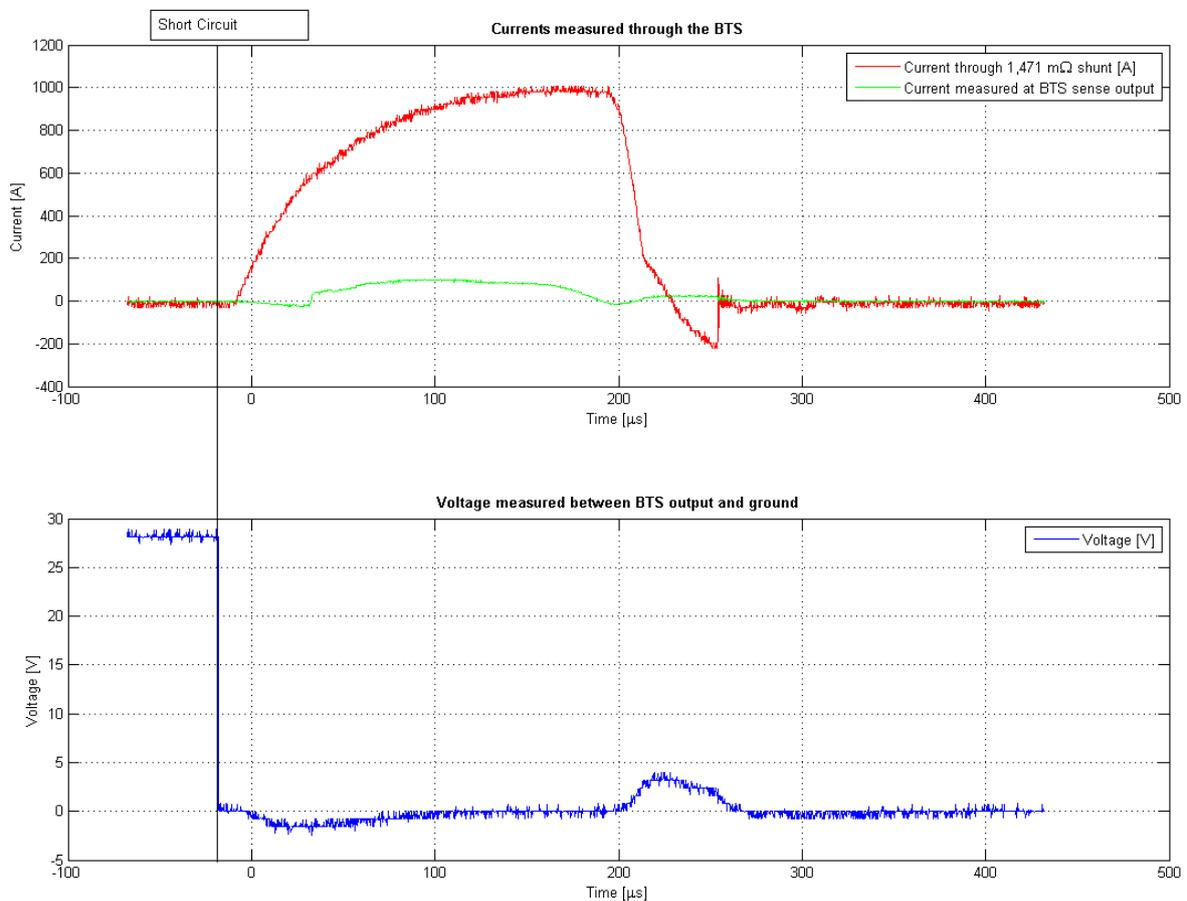
Figure 34: Short circuit testing of BTS555
