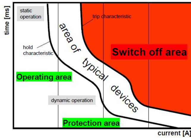
Figure 8: Internal tripping characteristic for a PROFET [22]
