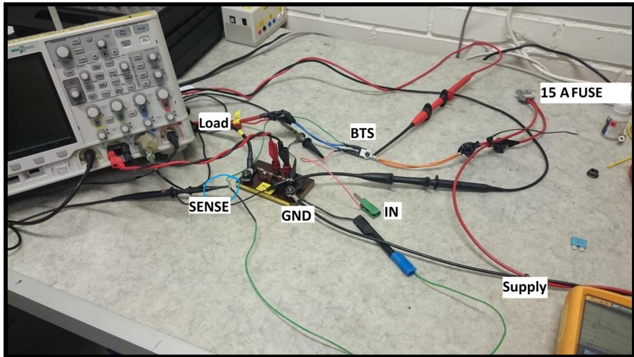
Figure 33: Setup for evaluating the BTS555
