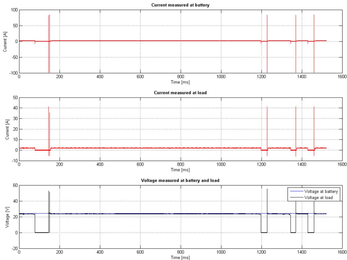
Figure 23: Currents and voltages measured when exposing a cable to bending
