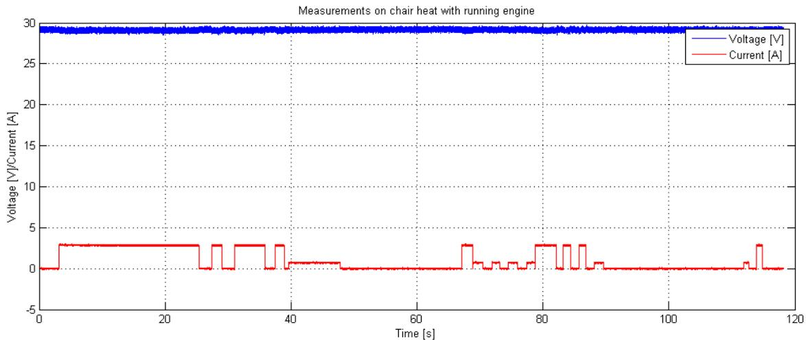
**Figure 12: Voltage and current measured at the chair heating fuse**
