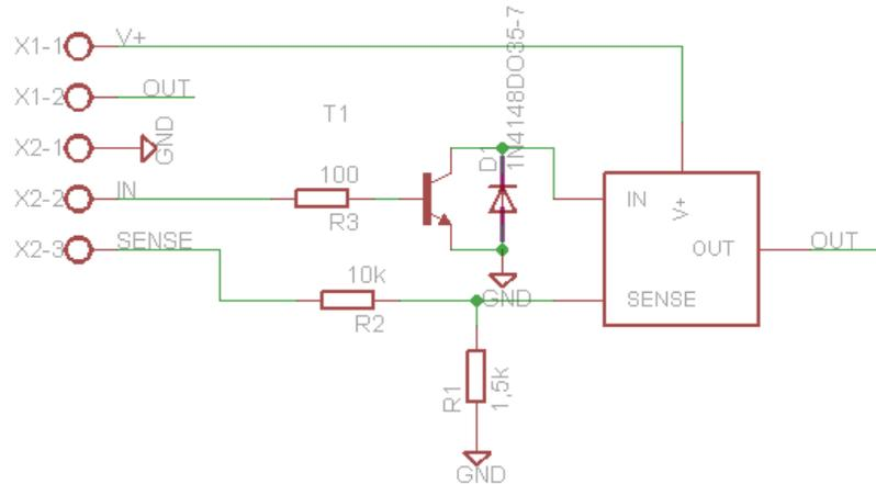
Figure 37: Schematic for an AUIPS7125 test board
