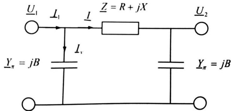
Figure 10: Medium length cable model [23]
