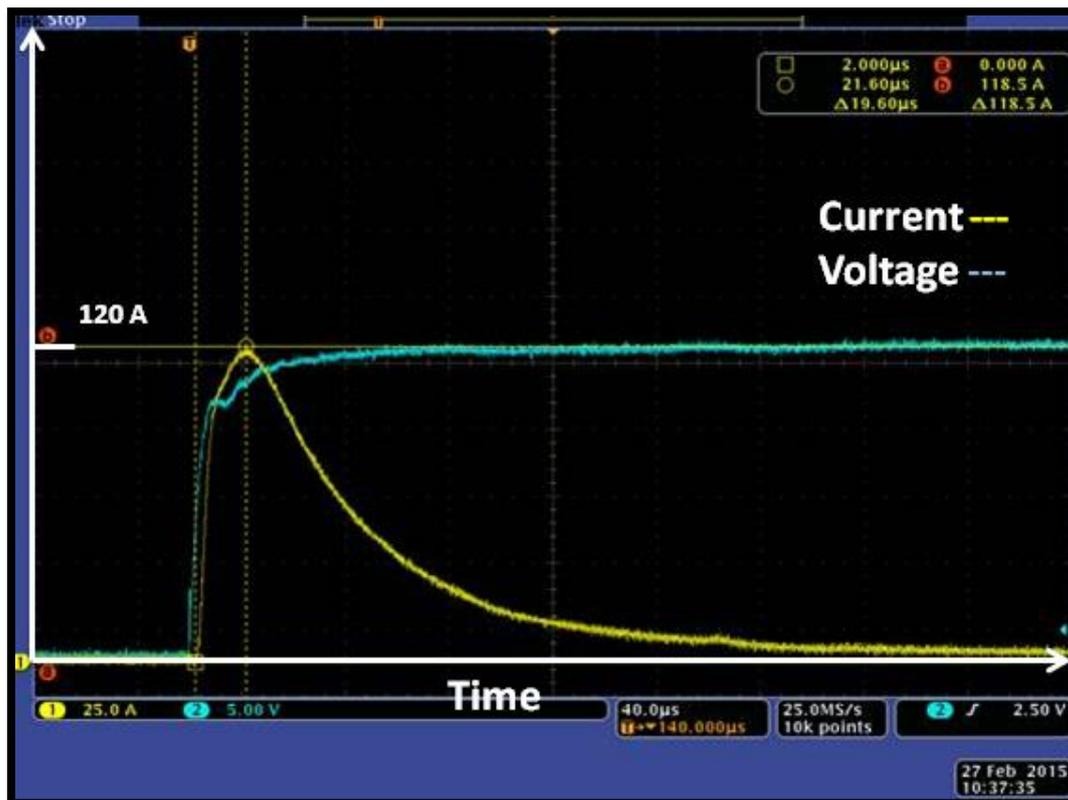
Figure 27: Current and voltage measurement performed on a component with severe inrush current and bypassed fuse
