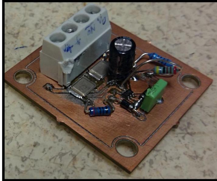
**Figure 36: Circuit for evaluating anti-serial MOSFETs**
