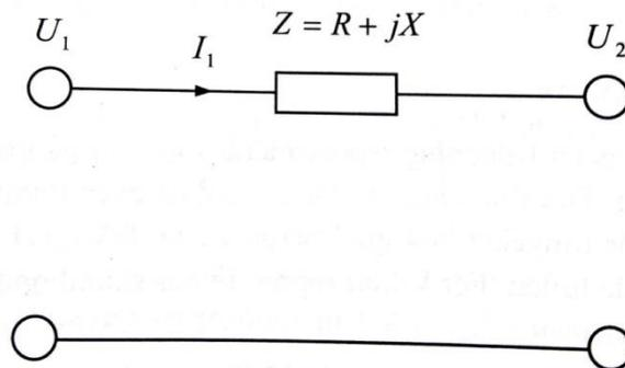
Figure 9: Short length cable model [23]
