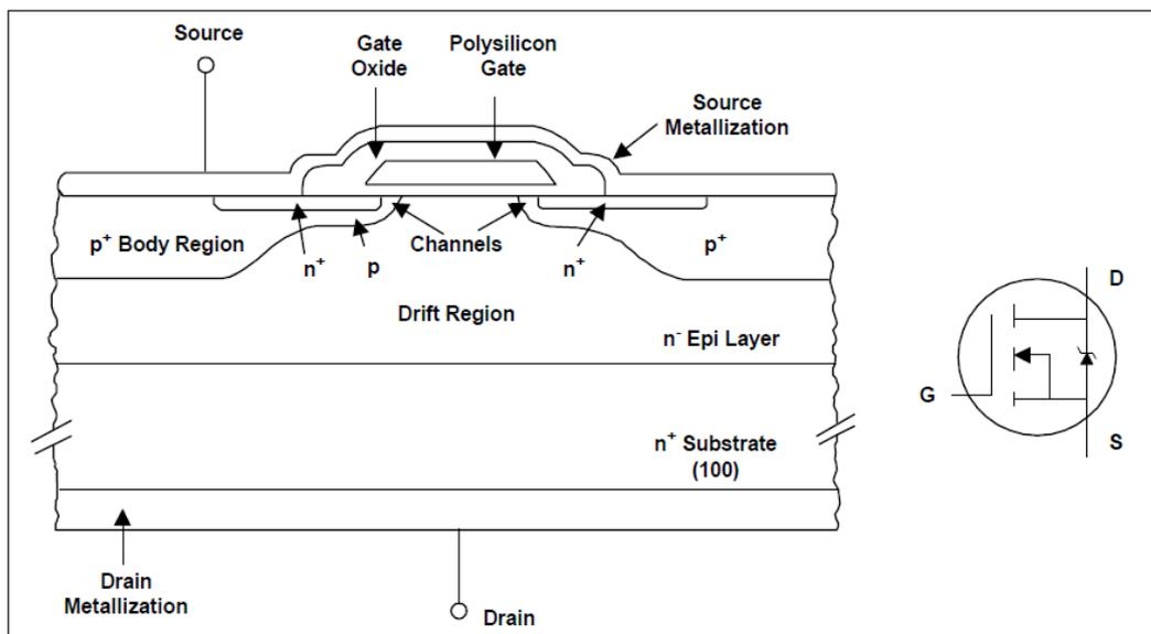
Figure 3: Structure and symbol of the n-channel MOSFET [10]
