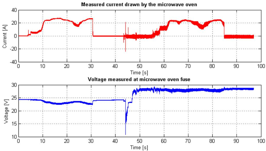
**Figure 13: Current and voltage measured at the microwave-oven's point of connection**
